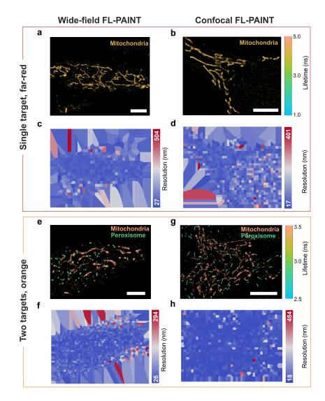
Figure S7: Image resolution estimation and FRC maps. Single-target wide-field (a) and confocal (b) FL-PAINT images of mitochondria. Lifetime colorbar is shown on the right-hand side of the images.(c-d) FRC maps of the corresponding super-resolution images from (a-b). The color bar on the right encodes the FRC resolution. Double-target wide-field (e) and confocal (g) FL-PAINT images of mitochondria and peroxisomes and corresponding FRC maps (f-h). Scale bars are 5 µm.
