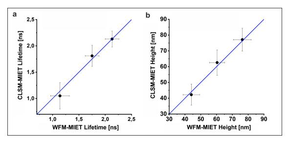
Figure S6: Comparison of average lifetimes (a) and heights (b) for wide-field and confocal MIET-SMLM measurements.
