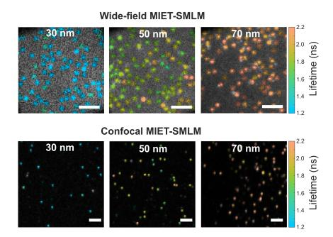
Figure S5: MIET-SMLM images of Cy3B fluorophores on top of a glass/gold/SiO<sub>2</sub> substrate for different values of SiO<sub>2</sub> layer thickness (30, 50, and 70 nm) for wide-field (top) and confocal (bottom) MIET-SMLM measurements. Scale bars are 1  $\mu$ m. The lifetime scale is shown on the right-hand side. Colors represent lifetime values.
