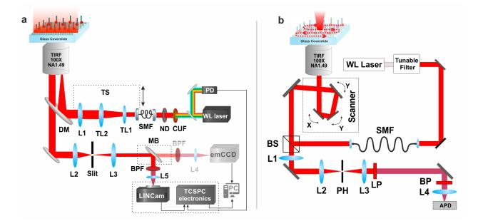
Figure S1: FLIM setups. Schematic representation of the custom-built wide-field FLIM setup equipped with lifetime camera (a) and time-resolved confocal FLIM setup equipped with fast scanner (b).
